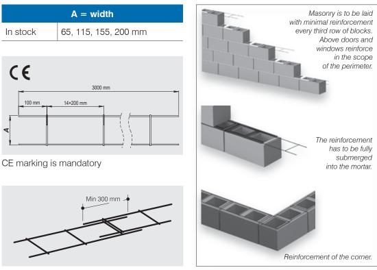
Overlapping when jointing min 300 mm
